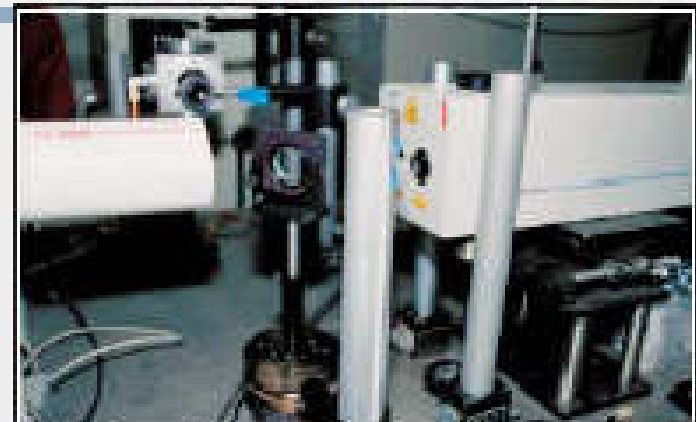
Experimental setup showing the target chamber and the LIBS laser
