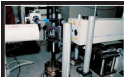
Experimental setup showing the target chamber and the LIBS laser
