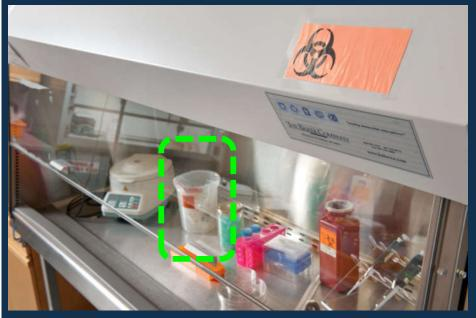
Use contaminated container in Biological Safety Cabinet to reduce drips to the biohazard bag
